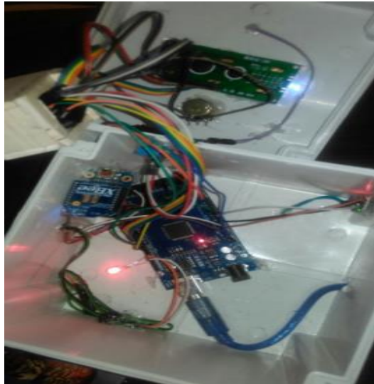
Figure 13. Arduino Xbee connection.
