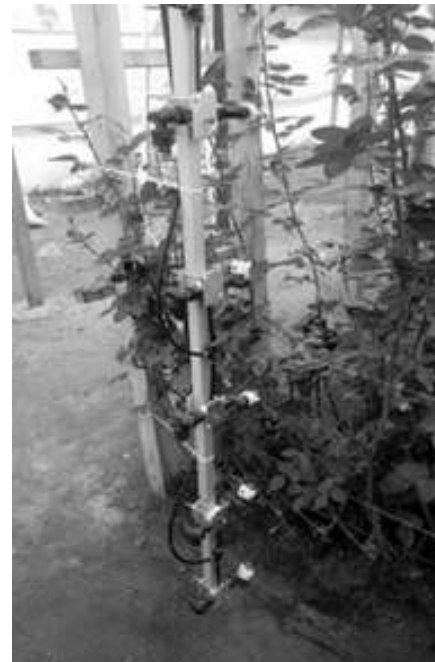
Figure 4. Detail of the boom construction with the sprinkler assembly installed. Source: own.
