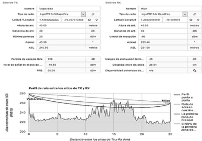
Figure 7. Radio link simulation between Valparaíso and Milán villages. Source: Ligocalc web.
