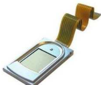
Figura 3. Lector de huella dactilar (ShenZhen Sanneng Security Technical, 2010).
