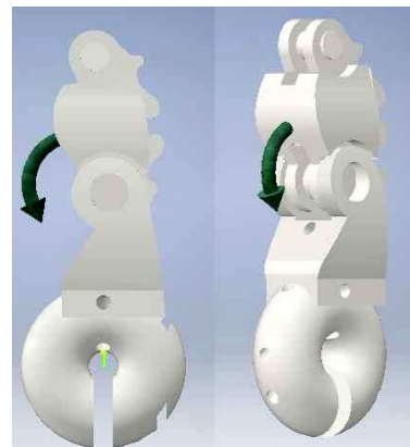
Figure 18. Movement of the joint of the middle and proximal phalanges.
