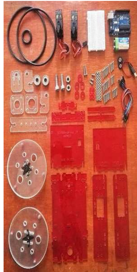
Figure 13. Parts of the robot's mechanical structure cut from acrylic sheet.
