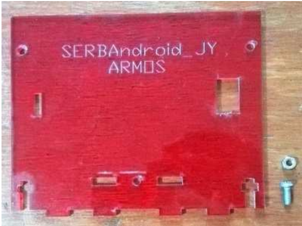
Figure 27. Rear face of the support structure for the smartphone.
