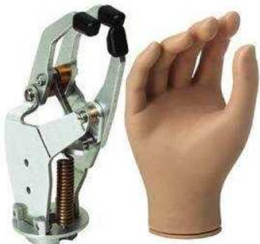
Figure 1. Electrically active hand prosthesis in the form of a clamp or hook.
