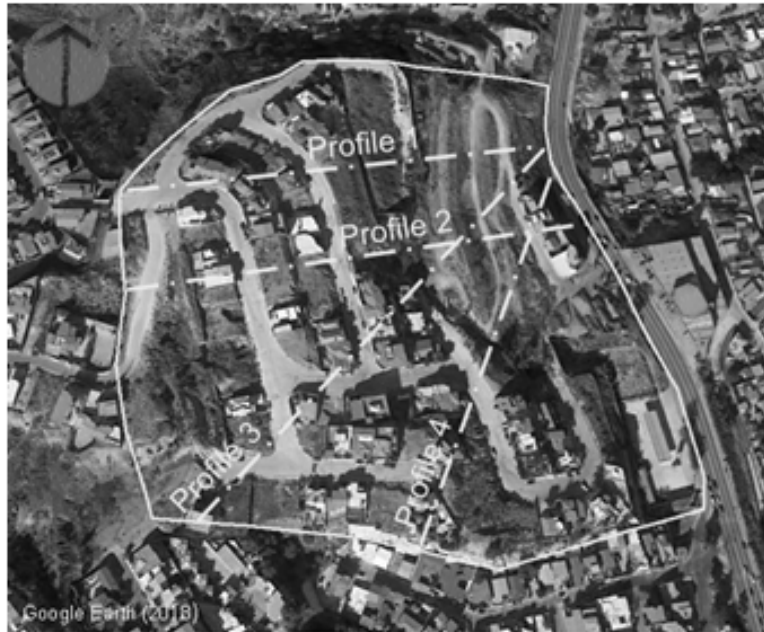
Figure 6. Profiles used for slope stability analysis.
